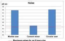
Figure 1 - Noise values obtained for the three positions analyzed compared with the limit of the standard NR-15 for unsanitary 85dB (A).
