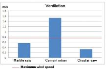
Figure 3 - Wind speeds obtained for the three working areas analyzed.
